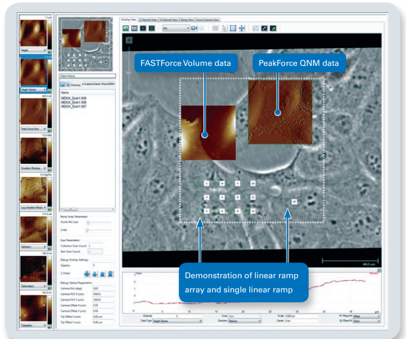
MIROView GUI enables seamless mode switching and automated measurements of multiple data types.
